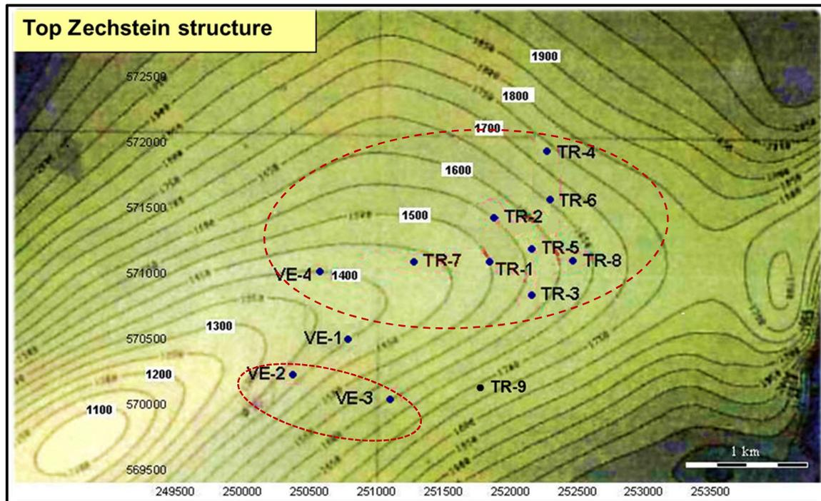
Positions of the 4 VE-wells (WHC-1) and 9 TR-wells (WHC-2), projected on top of the Zechstein (ZE) structure.
