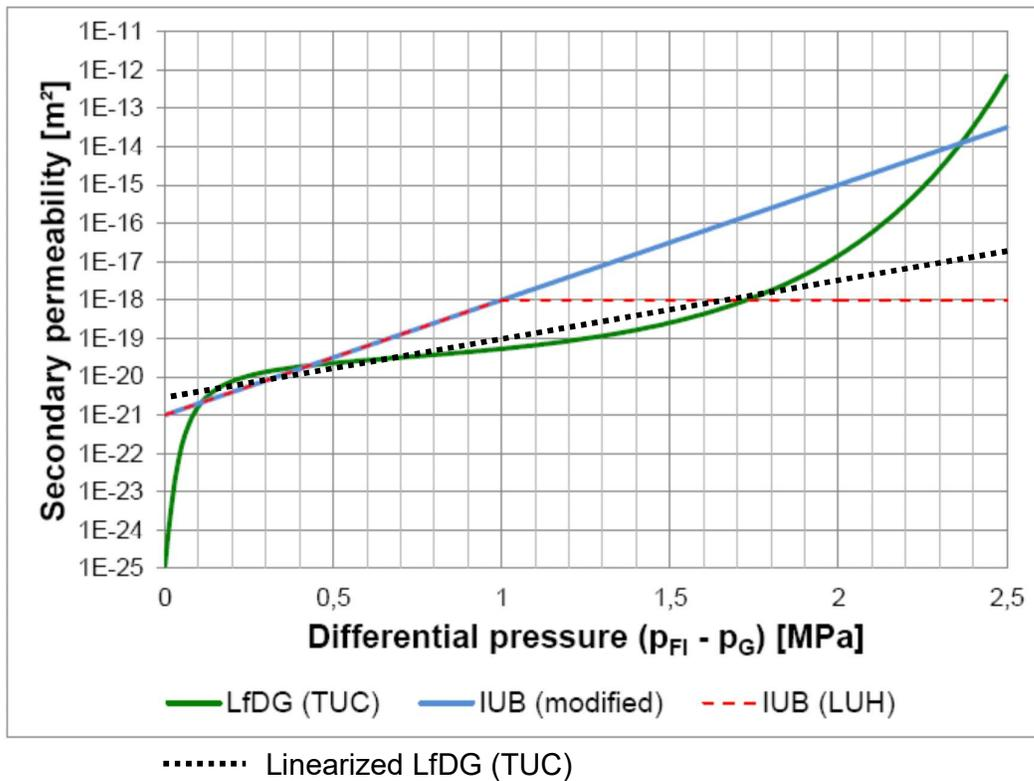
Different functional relations between effective brine pressure  $\sigma_e$  (= Differential pressure) and increase of salt permeability K (= Secondary permeability). The IUB modified curve has been applied in a Nedmag abandonment study (ref.2). In a new abandonment study (ref.4), a linearized version (dashed black curve) of the LfDG (TUC) curve is used.
