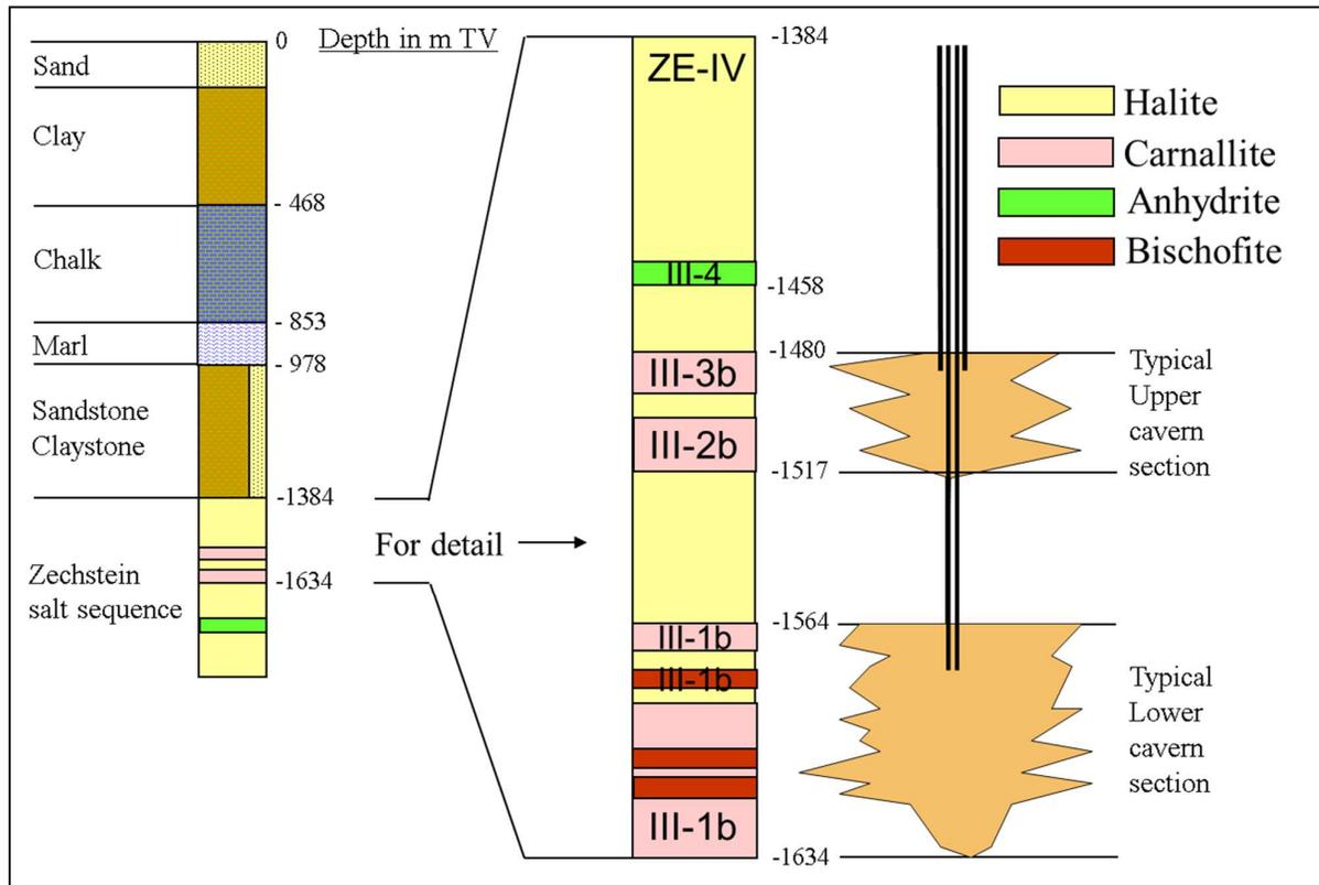
The magnesium salt extraction from the planned caverns VE-5 and VE-6 will only be performed in the Zechstein III-1b carnallite/bischofite sequence.
