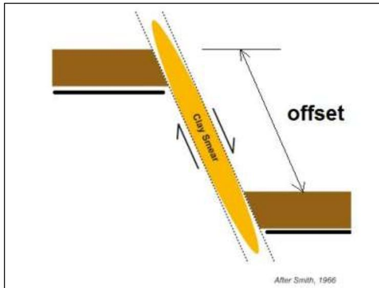
Schematic normal fault in impermeable rock (brown-colored), with offset larger than rock layer thickness. If the fault is sufficiently filled with clay smear (yellow colored), the fault is likely impermeable for hydrocarbons due to high capillary resistance. Then, if fluid lighter than pore water is trapped under the impermeable rock layer at the left side of the fault, the fluid cannot flow into porous permeable rock at the right side of the fault.
