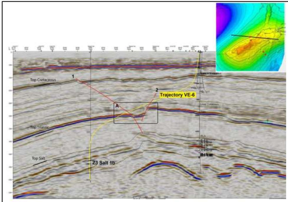
Right upper corner: Veendam salt pillow depth contour map, with cross section projected on map. Cross section shows well trajectory VE-6 (yellow line) with major faults in zone A.
