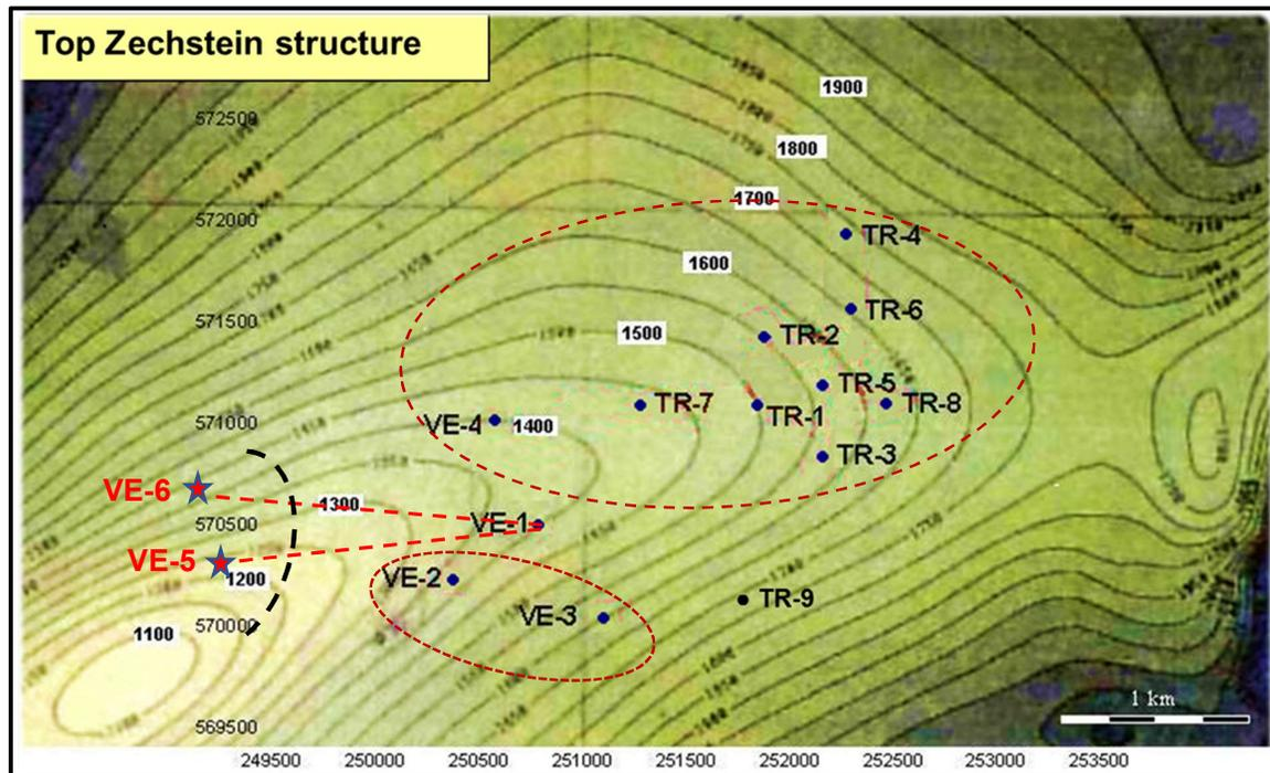
Nedmag well positions projected on top of the Zechstein (ZE) pillow structure. Positions of the planned wells VE-5 and VE-6 are indicated by red stars. The VE-wells are drilled from location WHC-1 located above well VE-1 (dotted trajectories). The black dotted curve is the expected leaching boundary in the direction of the other VE-wells.
