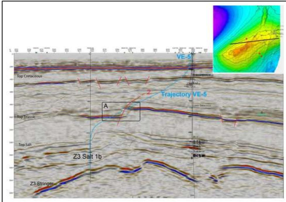
Right upper corner: Veendam salt pillow depth contour map, with cross section projected on map. Cross section shows well trajectory VE-5 (blue line) with major faults in zone A.
